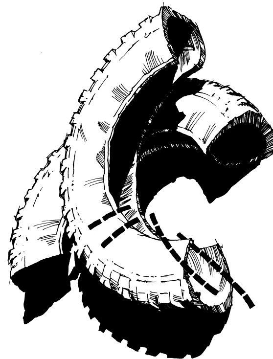
c. Cut a 3-inch triangle from each corner of one end of the sidewall.
